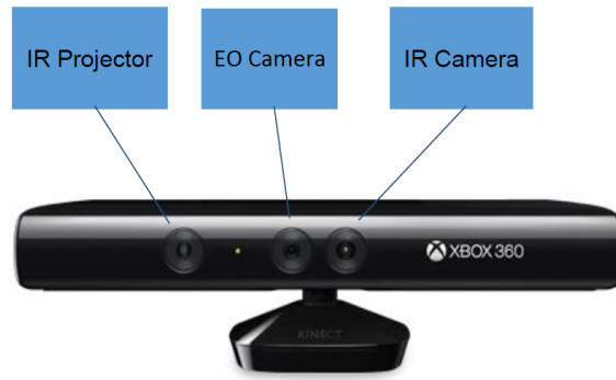
Figure 3: The Kinect Device having a built-in camera, sensors and features.
