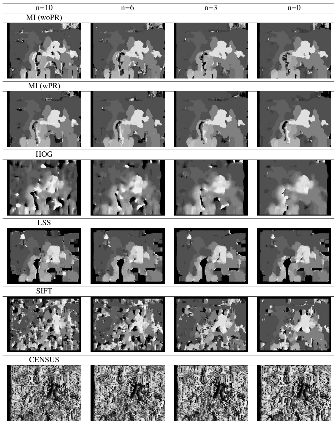
Figure 13: Sample visual results of some similarity measures for the added noise levels to Tsukuba left image in Dataset #1 (local window size=21x21) (noise levels: n = 10, n = 6, n = 3 and noiseless n = 0 )
