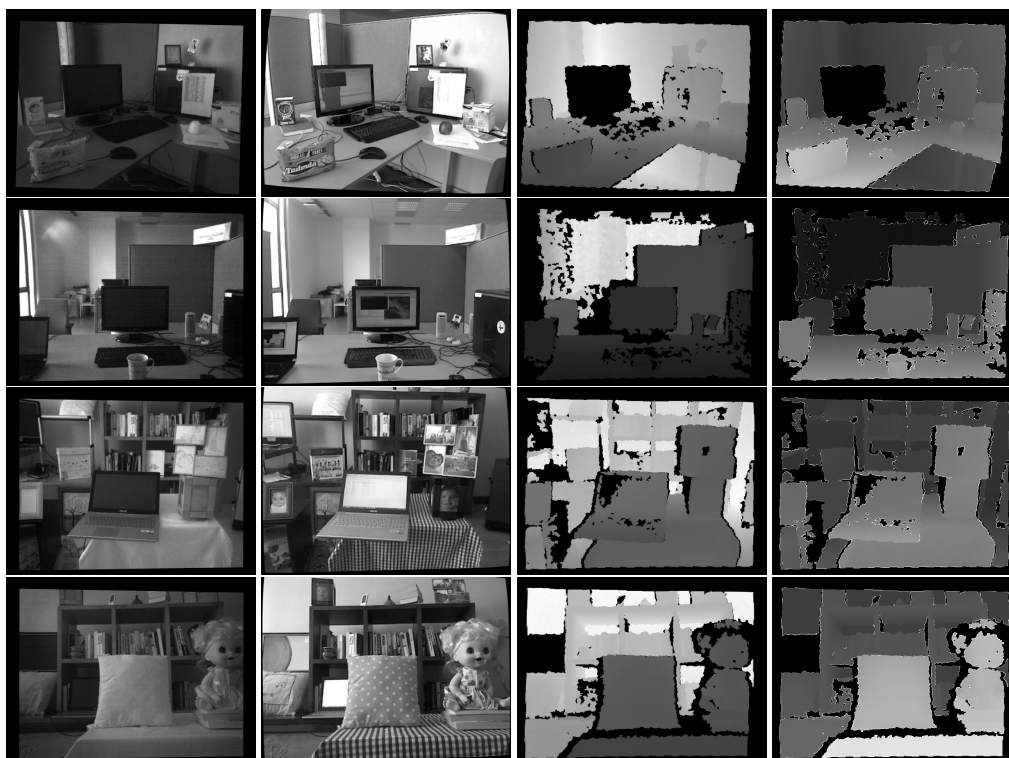
Figure 5: Sample image pairs from Dataset #2 - Kinect Dataset 1st column : Left (IR) camera images. 2nd column : Right (EO) camera images. 3rd column : Kinect's native depth maps (brighter pixels have more depth). 4th column : Disparity maps
