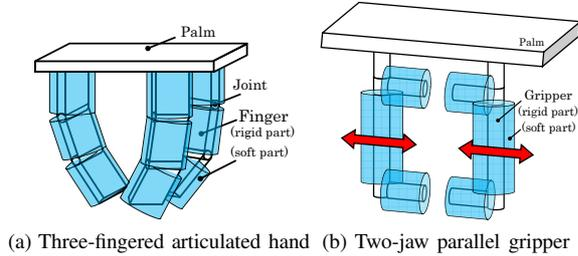
(a) Three-fingered articulated hand (b) Two-jaw parallel gripper
