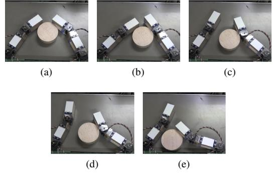
Fig. 5: In-hand caging manipulation (top-to-left)
