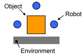
Fig. 1: Caging an object by robots and a wall
