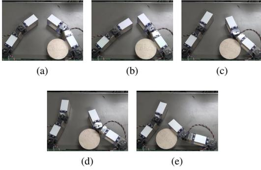
Fig. 4: In-hand caging manipulation (right-to-left)
