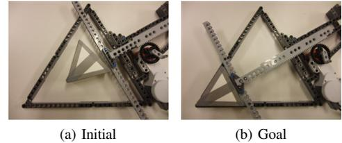
Fig. 7: 1-DOF hand for triangular objects
