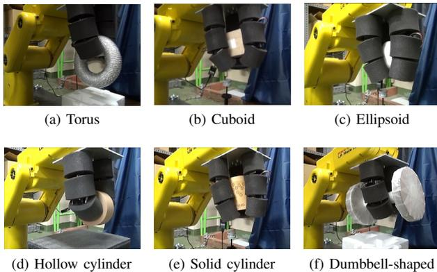
Fig. 10: Caging-based grasping by a two- or three-fingered articulated hand
