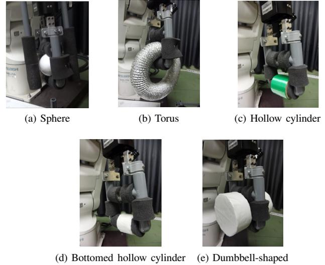
Fig. 11: Caging-based grasping by a two- or four-jaw gripper
