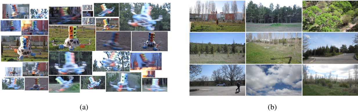
Figure 9. Example images from outdoor (a) quadrotor and (b) background training image sets. The images are colored, however their grayscale versions are used in the training. For quadrotor images, mostly the challenging examples are included.
