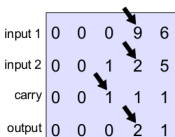
(a) Example scratch pad and pointers used for computing “ 96 + 125 = 221 ”. Carry step is being implemented.
