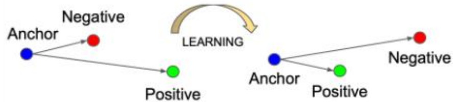
Fig. 1. Illustration of triplet loss given one positive and one negative per anchor. (Image source: Schroff et al. 2015 )
