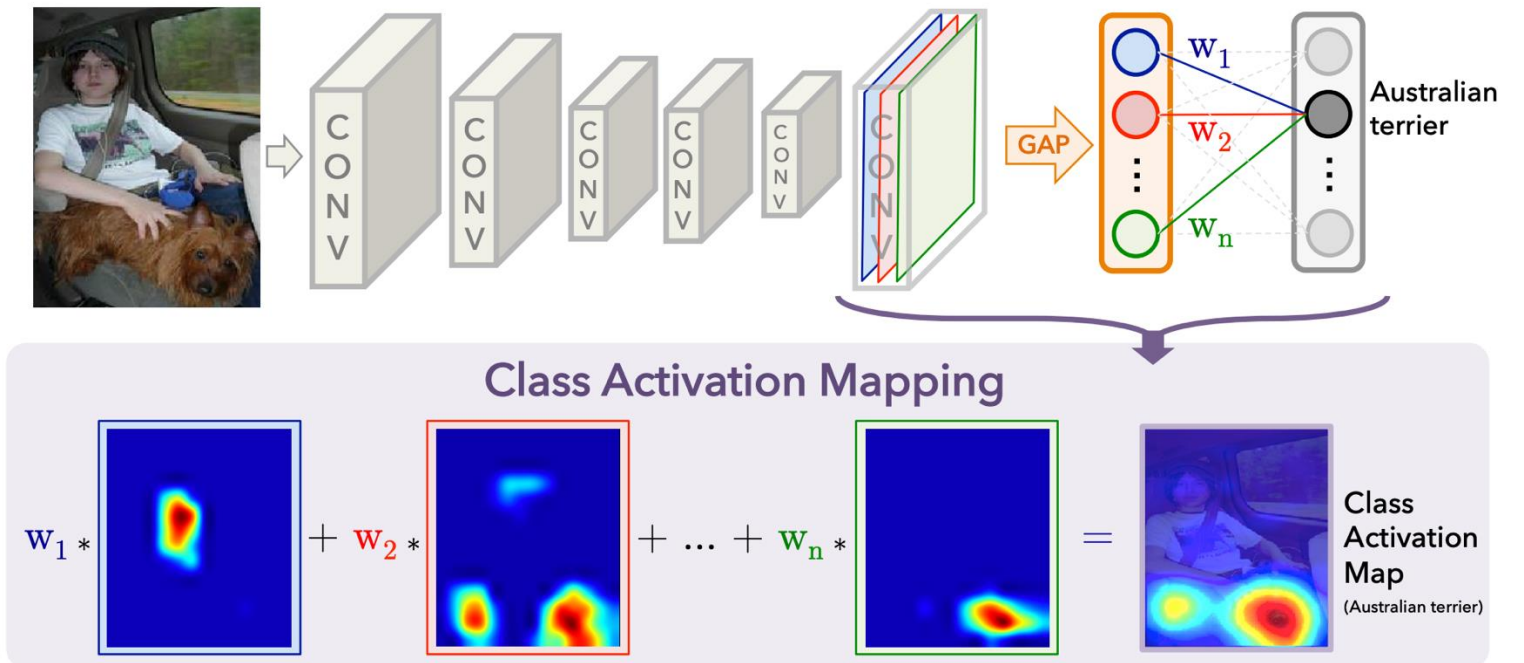
Figure 2. Class Activation Mapping: the predicted class score is mapped back to the previous convolutional layer to generate the class activation maps (CAMs). The CAM highlights the class-specific discriminative regions.
